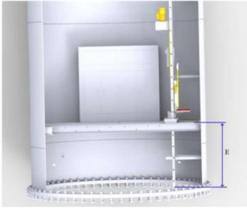
The top anchor point of the existing cable type fall protection system on the ladder is removable. Height of the top portion of the ladder above the top platform, G: 920 mm
