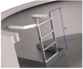
The top anchor point of the existing cable type fall protection system on the ladder is removable. Height of the top portion of the ladder above the top platform, G: 935 mm
