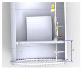
Ladder height under the starting platform, E: 1,700 mm
